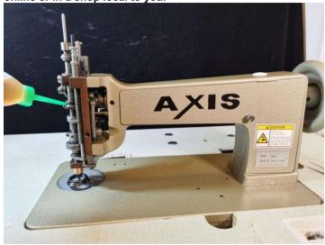
It is crucial to oil machine properly before each use! Refer to manual to see list of all spots to be oiled! Pictures above and below display two very important spots that should be oiled regularly!
