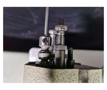
Picture bellows showing needle hook in 6 o clock position (facing same direction as handle crank)
