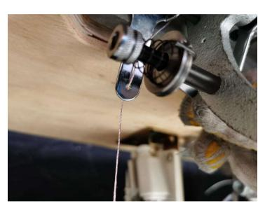
Thread should be fastened into wheel and secured under pin as shown below.
