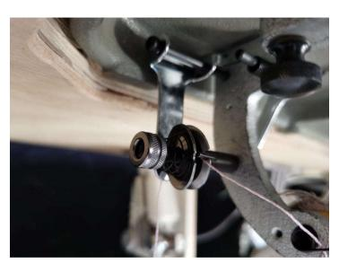
Pull a little bit of thread through loop to create a tiny bit of tension. this will allow wire threader to easily grab thread into machine!
