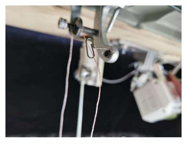
Pictured above, you can see wire threader coming through bottom of machine to grab thread and pull it back up.
