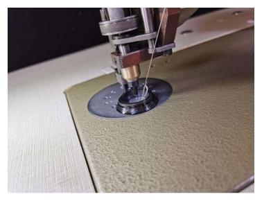
While holding the thread slightly with your left hand, at the same time, turn the handle wheel shown below with your right hand. this will drive needle downward to catch the thread and pull it up. Make sure machine is OFF and foot is not on foot pedal while threading machine!
