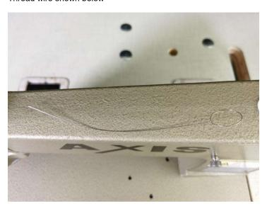
To thread machine, rotate the handle crank and look at the needle plate closely until you see a hole/opening to insert wire threader into machine to grab thread and pull back through.
