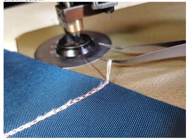
Trim the end of the thread, and tie off the end of the stitch as shown in the series of pictures below.
