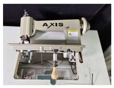
The screw of needle bar holder and needle hook and handle crank should be in the "6 clock direction", or facing user. This is an important step to properly setting up the machine! See pictures on next page below for reference!
