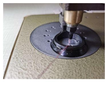
The needle will pull up the thread as shown above, and you will need to use tweezers to pull the thread out of the needle hole.
