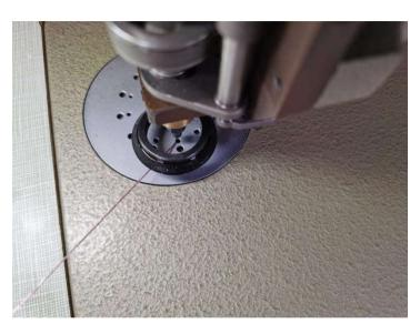
Switch on the motor, press down foot pedal, and rotate the handle crank direction to stitch as your desire! It is recommended to start on denim/jean fabric to practice. Using a lower weight thread will produce thicker and more textured stitching. Experiment with different thread weights to find the type you desire!
