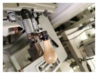
Picture below shows the stop motion rocker when it is pushed up/not ready to stitch. Get comfortable pulling and pushing handle crank, while looking at the inside of the machine to get a better understanding! And always keep your machine well oiled!
