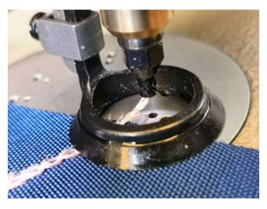
Using your tweezers, insert them into the middle of threads when the needle raised at the top. This is essentially undoing the loop from the needle hook and keeping tweezers inside of that hole
