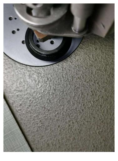
Once you have found and lined up the proper hole in the needle plate, Insert the thread wire into the needle plate hole carefully, and then hook up the thread from end of tension spring as shown below
